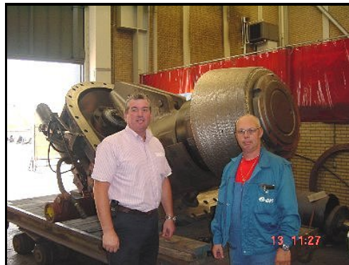
This is the ROTATING UNIT that crushes the coal.
