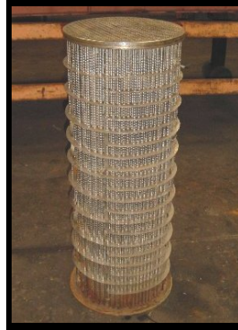
This is the nest from the Heat Exchanger Unit
