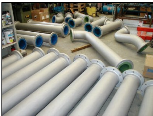
The pipes are 2 meters in length and have a 200mm internal bore.
